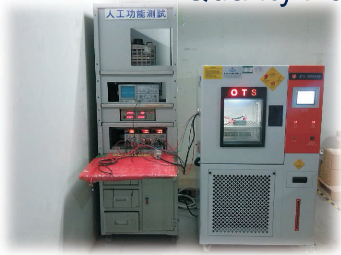
Temperature Humidity Chamber
