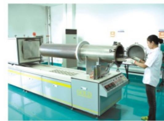
Nitrogen protection and vacuum-sintering
