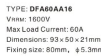
$I_d=30A \sim 500A$ ,  $I_{jm}=125^\circ C$ ,  $V_{DRM}=V_{RRM}=1600V$  or custom made,  $V_{ISO} \geq 2.5KV_{(RMS)}$
